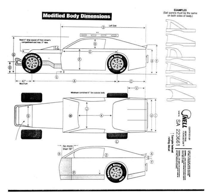
Rear bumper must resemble one of the following designs. (A) Solid bumper of square or round tubing, no wider than five inches outside each rear frame rail. (B) If rear bumber is wider than five inches outside rear frame rails, it must be capped, with no sharp edges, and bent forward on the ends at a 90 degree angle. (C) A bumper constructed in a loop design.
